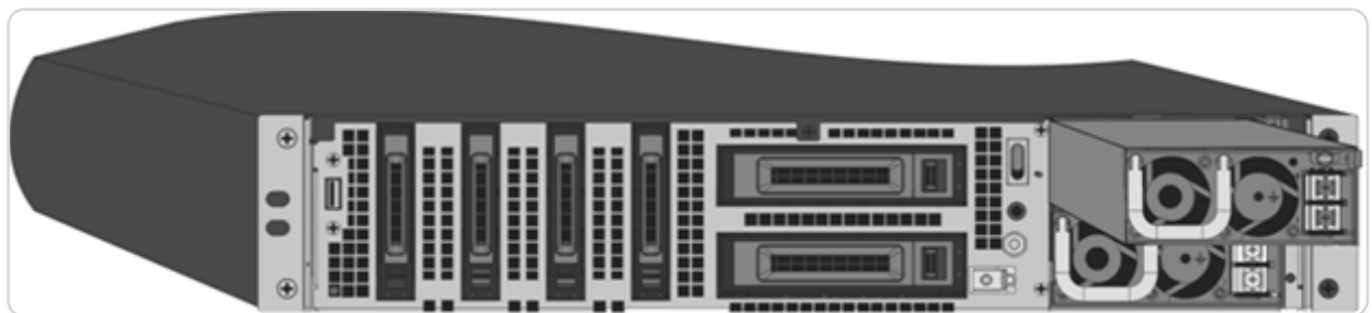
Figure 4. Insert the Replacement DC Power Supply
