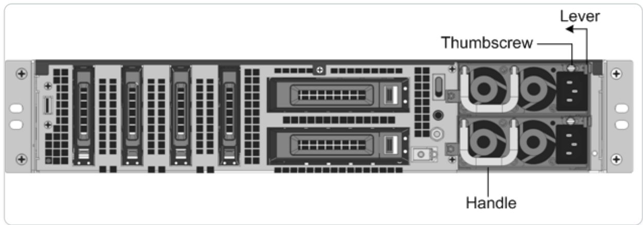
Figure 2. Remove an Existing DC Power Supply
